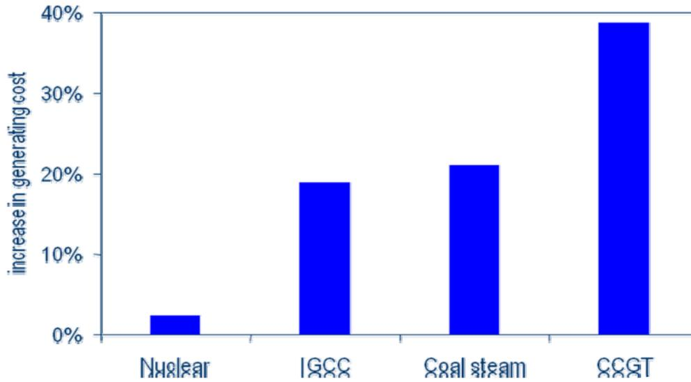
Figure 3: Impact of 50% increase in fuel cost on generating cost, new plants
