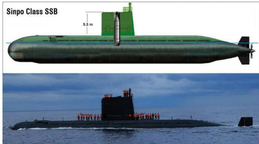
Figure 4: DPRK *Sinpò* Class ballistic missile submarine
