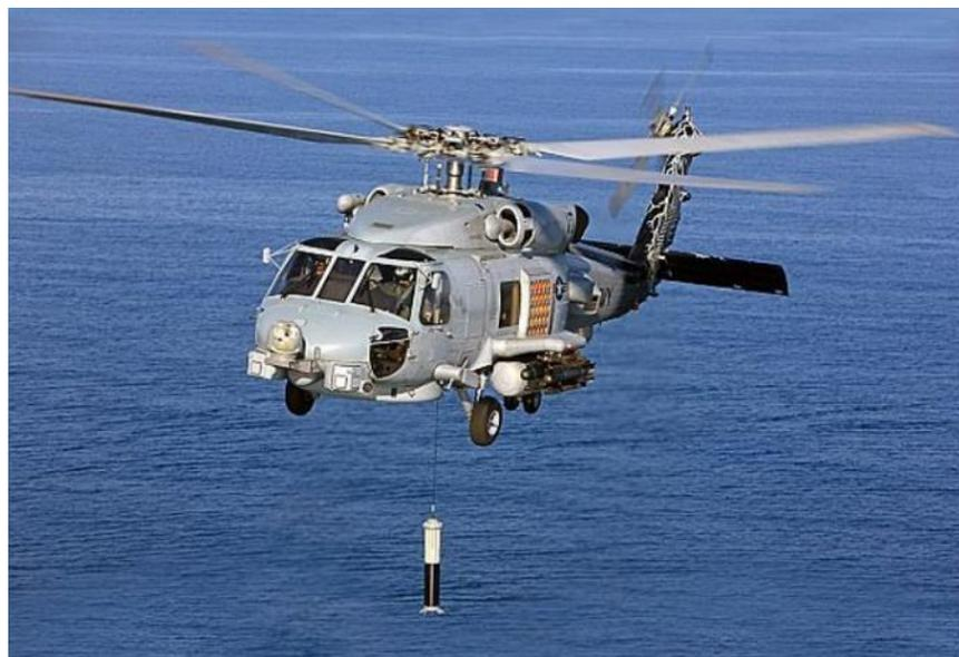
Figure 4: MH-60R deploying dipping sonar
