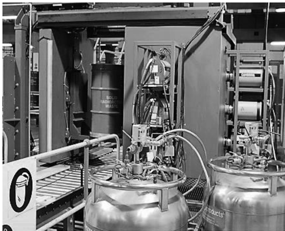
Figure 9-3. IQ 3 Scanner Used for Verification of Uranium in Waste Drums. 9
